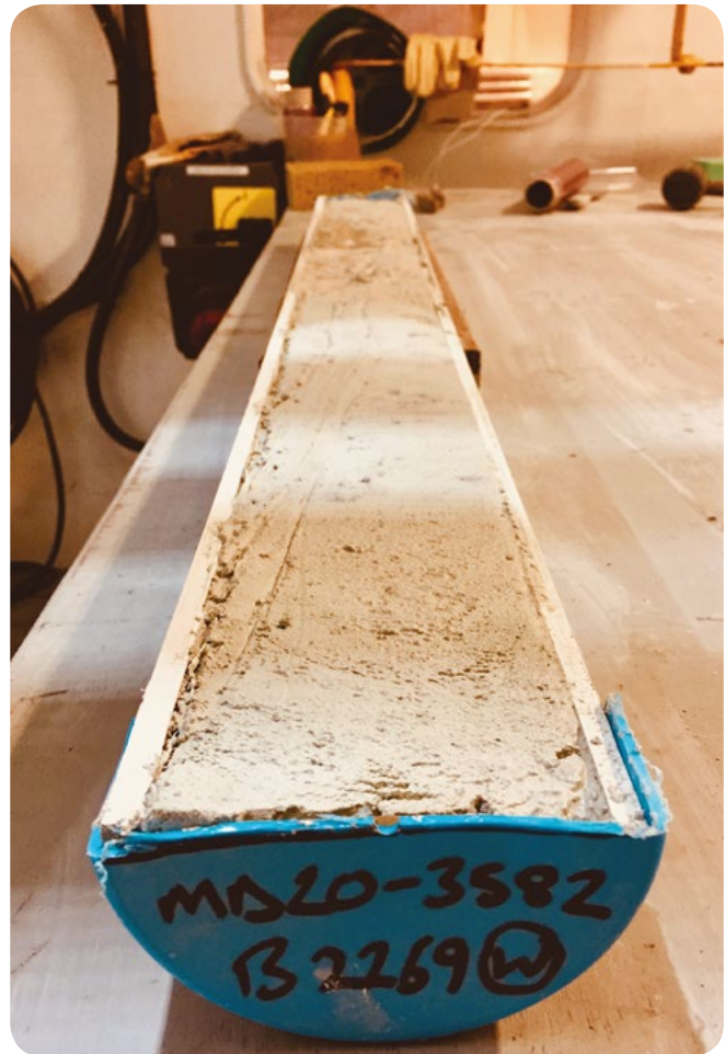
ON THE ACCLIMATE-2 CRUISE, THE CALYPSO CORER COLLECTED EIGHT LONG SEDIMENT CORES, INCLUDING FOUR THAT WERE 60 M LONG AND IN EXCELLENT CONDITION. © UB/María de la Fuente
