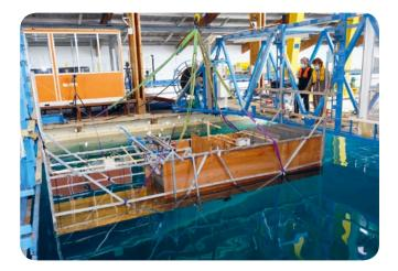
HYDRODYNAMIC TESTS BEING PERFORMED IN THE TANK AT IFREMER'S CENTRE DE BRETAGNE, WHICH HAS BEEN MADE AVAILABLE FOR TESTING THEOREM PROJECTS AT EVERY STAGE OF DEVELOPMENT, FROM PROOF OF CONCEPT THROUGH INDUSTRIALIZATION. © Ifremer / Olivier Dugornay
