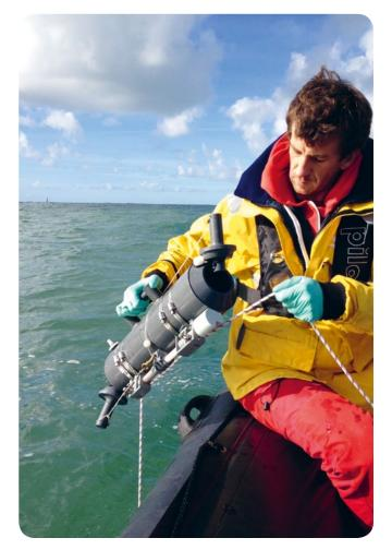
SAMPLING NEAR THE MOUTH OF THE LOIRE FOR A REPHY OBSERVATION STATION THAT WILL HELP MONITOR PHYTOPLANKTON NUMBERS AND MEASURE OTHER ASPECTS OF THE WATER COLUMN (TEMPERATURE, SALINITY, DISSOLVED OXYGEN AND TURBIDITY). © Ifremer
