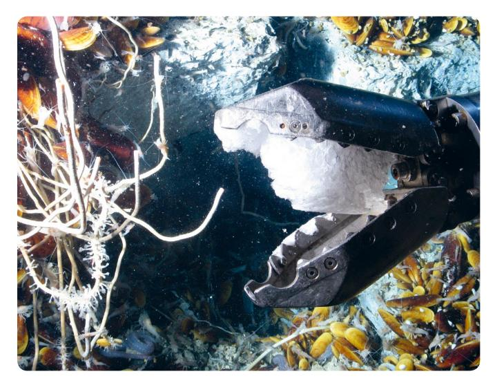
REMOTELY OPERATED SUBMERSIBLE VICTOR 6000 GRIPS A CHUNK OF GAS HYDRATE, THE MYSTERIOUS "ICE THAT BURNS." © Ifremer
