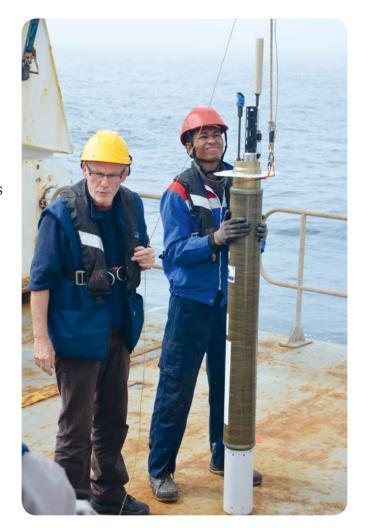
NEW AUTONOMOUS ARGO FLOATS, NOW SMARTER AND MORE DURABLE, DEVELOPED AS PART OF THE NAOS PROJECT (NOVEL ARGO OCEAN OBSERVING SYSTEM) CO-LED BY IFREMER AND SORBONNE UNIVERSITÉ © Ifremer / Kevin Balem
