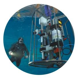
LAUNCHED IN THE FRAMEWORKOF THE EUROPEAN SEAFLOOR OBSERVATORY (EMSO), THE GENERIC INSTRUMENT MODULE (EGIM), DEVELOPED BY IFREMER, IS A STANDARDISED MEASUREMENT TOOL EMBEDDED WITH NUMEROUS SENSORS AND IS USED TO FIT SUBSEA OBSERVATION STATIONS. © Ifremer - O. Dugornay
