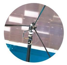
QUALIFICATION TRIALS FOR ROTOR PROTOTYPE IN TEST TANK AT IFREMER BREST © Ifremer - O. Dugornay
