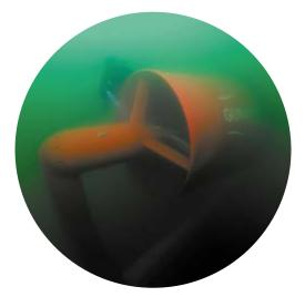
27 FEBRUARY 2019: SUBMERSION OF THE GUINARD ENERGIES P154 MACHINE IN THE ETEL RIA FOLLOWING POSITIVE TRIALS CONDUCTED IN JANUARY IN THE BAY OF BREST. THIS 20KW TIDAL STREAM TURBINE, DEVELOPED IN THE FRAMEWORK OF THE MEGAWATTBLUE PROJECT (GUINARD ENERGIES/IFREMER/ENSTA PARTNERSHIP), WAS SET UP ACCORDING TO PLAN AND WILL BE CONNECTED TO THE GRID VERY SOON. CURRENTLY, THE TURBINE IS OPERATING AND IS BEING VALIDATED. © Ifremer - O. Dugornay
